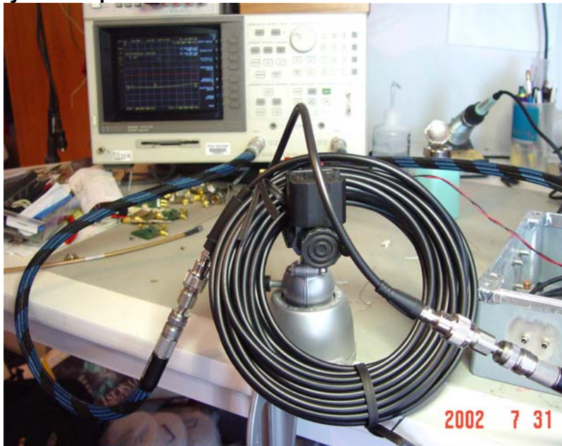
Figure 16. 15.2 meter / 50 foot section of commercial 75 ohm RG-6 coaxial cable being tested. Note measurement system impedance is 50 ohms.
